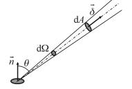
• The radiative spectral intensity noted  $I_{\lambda}$  is the energy emitted by a surface per unit surface normal to the rays, per unit of time, per unit of solid angle and per unit of spectral range
