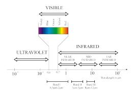
Thermal radiation is defined to be those electromagnetic waves which are emitted by a medium due solely to its temperature. The associated spectral tange i between 0.1 µm and more than 100 µm.
