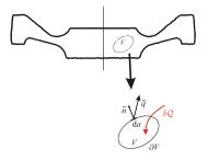
If we postulate the local equilibrium of this volume, the application of the first law of thermodynamics between time t and time  $t + \mathrm{d}t$  for a transformation at pressure volume gives:
