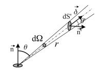
This transfer can be compared to the total radiated pover leaving dS:
