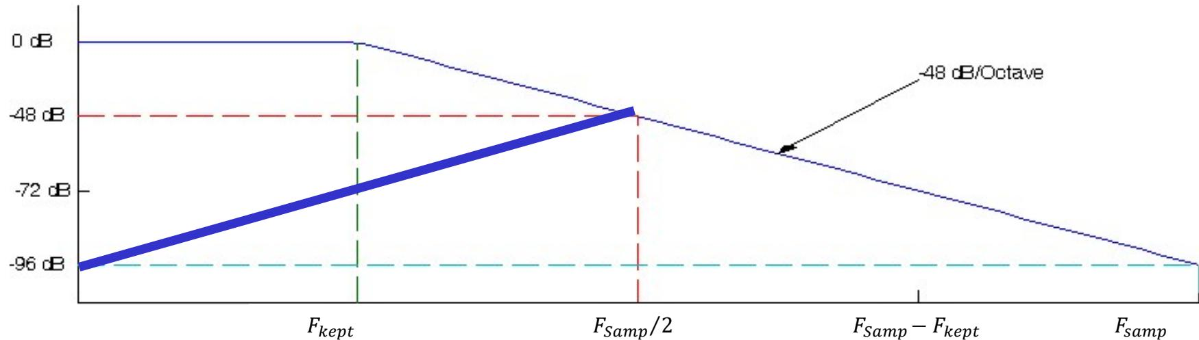
Objective : **aliased signal** reduced by resolution at  $F_{kept} = F_{sample}/(2+\alpha)$
