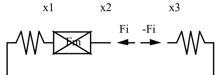
Internal force application  $\Rightarrow$  improper test
