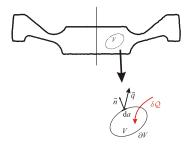
If we postulate the local equilibrium of this volume, the application of the first law of thermodynamics between time t and time t + dt for a transformation at pressure volume gives:
